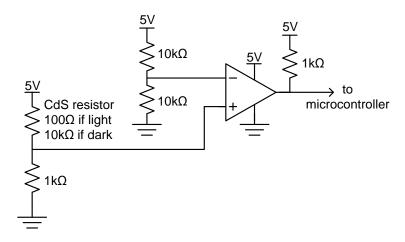
It works well when exposed to sunlight and in an office lit by incandescent light, but works unreliabily in an office lit by fluorescent lights.
