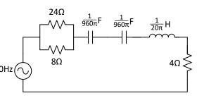
a) Find the real power P and complex power **S** power delivered to the  $4\Omega$ resistor.
