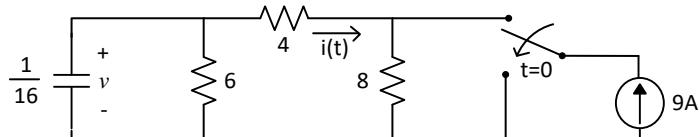
$t < 0$  (find  $V_0$ ) To find  $V(t)$  must first find  $V_0$ ,  $V_\infty$ ,  $\tau$ . To find  $i(t)$ , note  $i(t) = \frac{V(t)}{4+8}$
