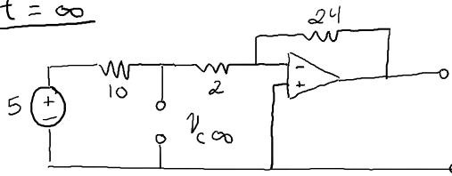
$$\text{KCL at } V_c: \frac{V_c - 5}{10} + \frac{V_c - 0}{2} = 0 \Rightarrow V_\infty = \frac{5}{6}$$
