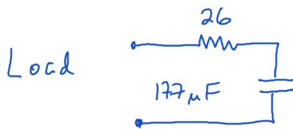
$$\left. \begin{aligned} \frac{-j}{\omega C} &= -j15 \\ \omega &= 2\pi 60 \end{aligned} \right\} C = 177 \mu F$$
