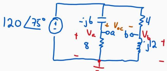
$$V_a = 120 \angle 75^\circ \frac{8}{8-j6} = 96 \angle 112^\circ$$
