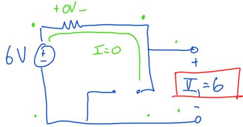
$$\begin{aligned} Z_C &= \frac{1}{j\omega C} = \frac{1}{j0 \cdot \frac{1}{10}} = \infty \\ v_1(t) &= 6V \end{aligned}$$
