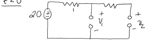
By inspection  $v_1 = v_2 = 20V$
