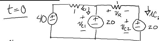
$$\begin{aligned}v_R &= 20 - 20 = 0V \\i_{C1} &= C v'_{C1} \\ \Rightarrow v'_{C1} &= \frac{1}{C_1} i_{C1} = (2)(20) = 40V/s \\ v_{C2} &= \frac{1}{C_2} i_{C2} = (3)(0) = 0V/s\end{aligned}$$
