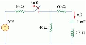
**P3** Find C in the circuit below so that the response is underdamped with a unity damping factor  $(\alpha = 1)$ .
