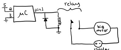
normally the diode looks like an open, until pin suddenly turns off. Then Upin < 0 and the diode becomes an open, keeping Upin from going much less than 0.
