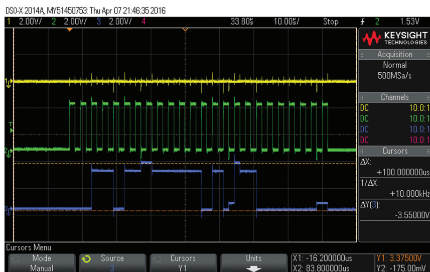
FIG2 The Wild West of FPGA design: A scope screenshot taken while debugging SPI communications errors. The blue channel should be a square wave showing data being sent from an external ADC to the MISO pin on the ARTY. The spikes on the channel suggest that the reference documentation for the software-designed SPI port have reversed the MOSI and MISO pin names, so the FPGA is attempting to (feebly) push data out on its input line. We assume reference documentation to be correct, but this scope capture shows that is not always the case.
