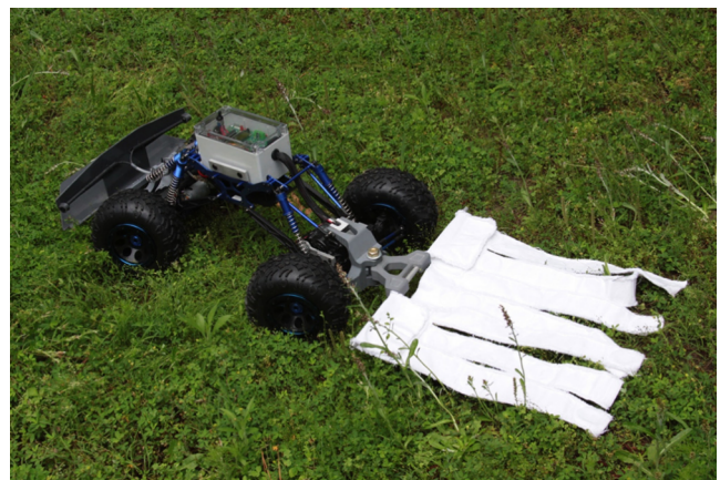
Fig. 1. Photograph of semi-autonomous robot (Tickbot 2) for killing ticks in vegetation. The robot navigates by following a magnetic signal transmitted along a guide wire placed along trails. The device drags a white denim cloth impregnated with an acaricide (see text for additional details).
