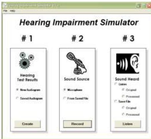
Figure 3: The Home screen is the hub for the Hearing Impairment Simulator user interface. All supporting screens return to the home screen.
